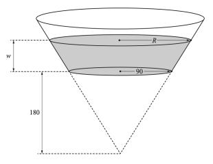
The diagram shows a large hollow cone from which a smaller cone of height 180 and base radius 90 has been removed. The remainder has been fitted with a circular base of radius 90 to form a container for water. The depth of water in the container is w and the surface of the water is a circle of radius R.
